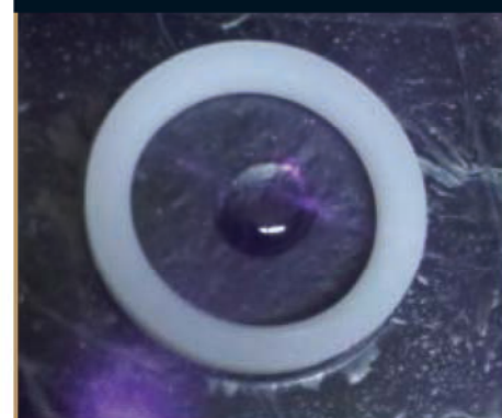
Human SC mounted on the sample holder on which a drop is applied.
