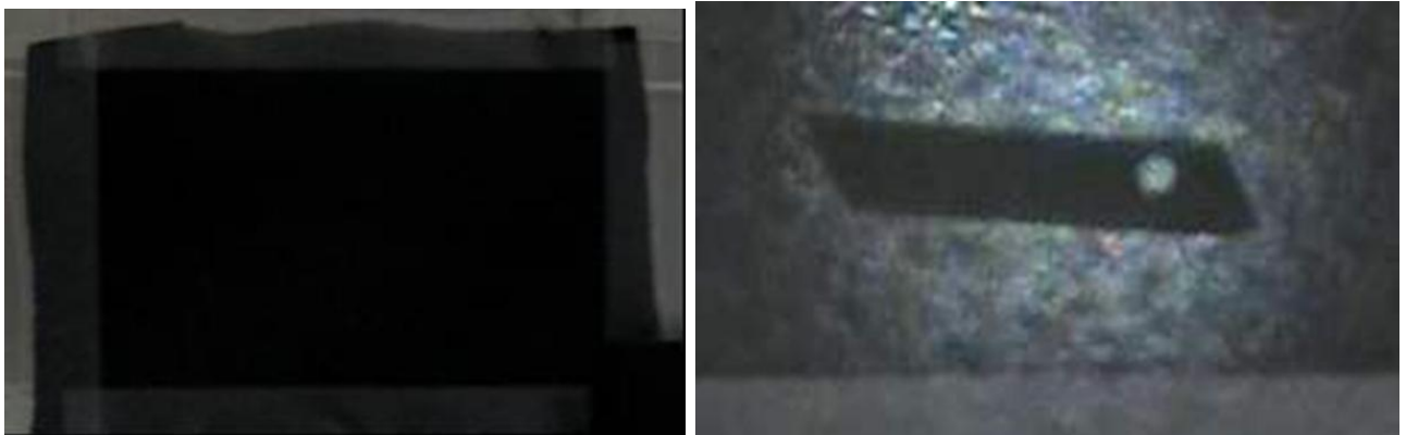
Fig. 4. A metallic knife hidden behind a thick dark cloth is revealed by the terahertz beam. Picture was taken in transmission.
